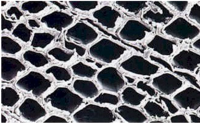
Photograph, taken through an electronic microscope, showing a section of a thin layer of fir wood-wool taken from a standard panel. University of Padua, February 1995.
