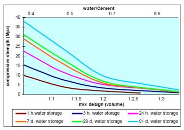
The data provided in the graph has been supplied by the Vicat Company, the manufacturers of Prompt as a guide to strength gain with the variables of water cement ratio and mix strength, and as such are relevant to the specific aggregates used.
