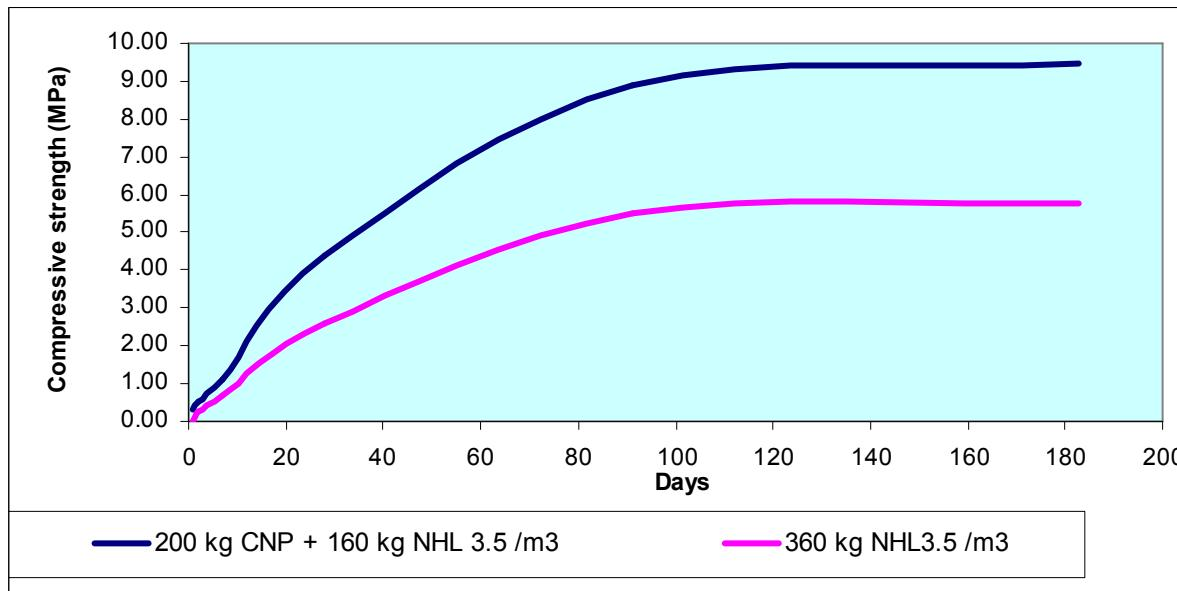
Although compressive strengths (Fig. 10) are higher with our mix than with the control mix, nearly the same elasticity modulus (Fig. 11) and a sharply lower drying shrinkage (Fig. 12) lend the present mix all sorts of durability guarantees as regards both bonding and cracking.
