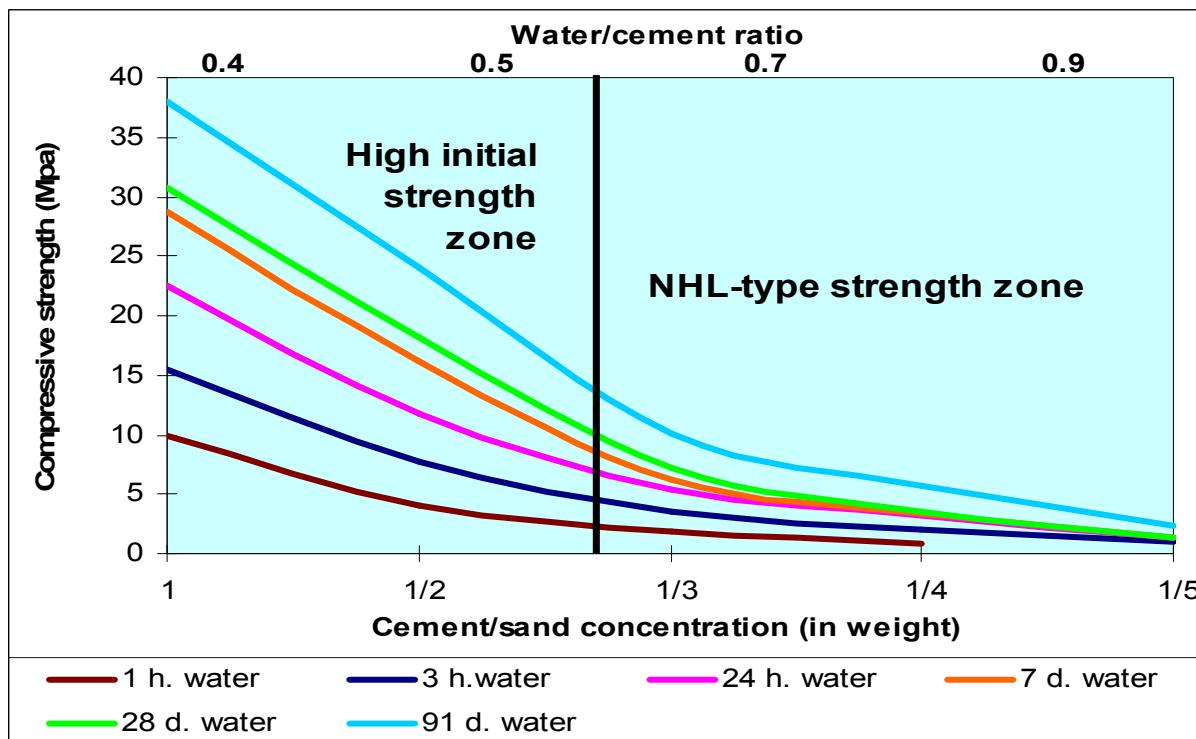
Whether with respect to the W/C ratio or concentration, PNC strength values can be categorized into two zones:
